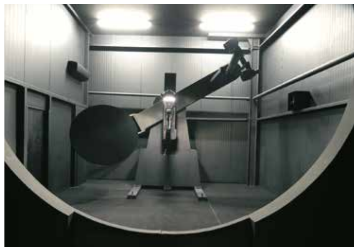
The most modern device to perform photometric tests in ROSA laboratory.
